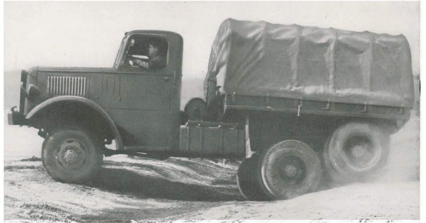
Macks are built to take the worst punishment the Army can hand out. Here, one of the big Mack prime movers hurtles across uneven ground at high speed—just one of the exhaustive tests to which these trucks were subjected before acceptance by the Army. Note the extreme flexibility of the rear bogie under this terrific strain.
