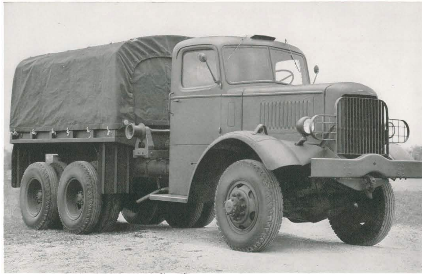
Biggest Trucks in Army service, each of these Mack prime movers has a gross weight of over 20 tons when fully loaded and pulling anti-aircraft gun.
