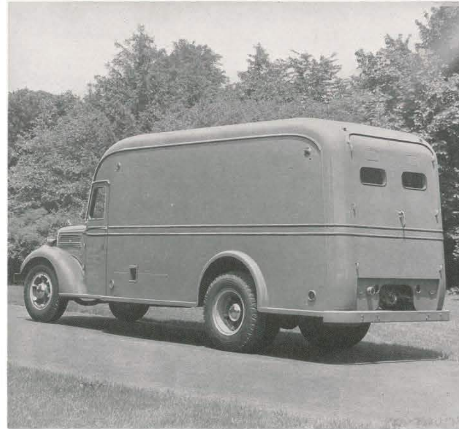
A Mobile Radio Station, this Coast Guard Mack carries a portable transmitter and receiver for use during floods and hurricane disaster, and for maintaining radio apparatus at various Coast Guard stations.
