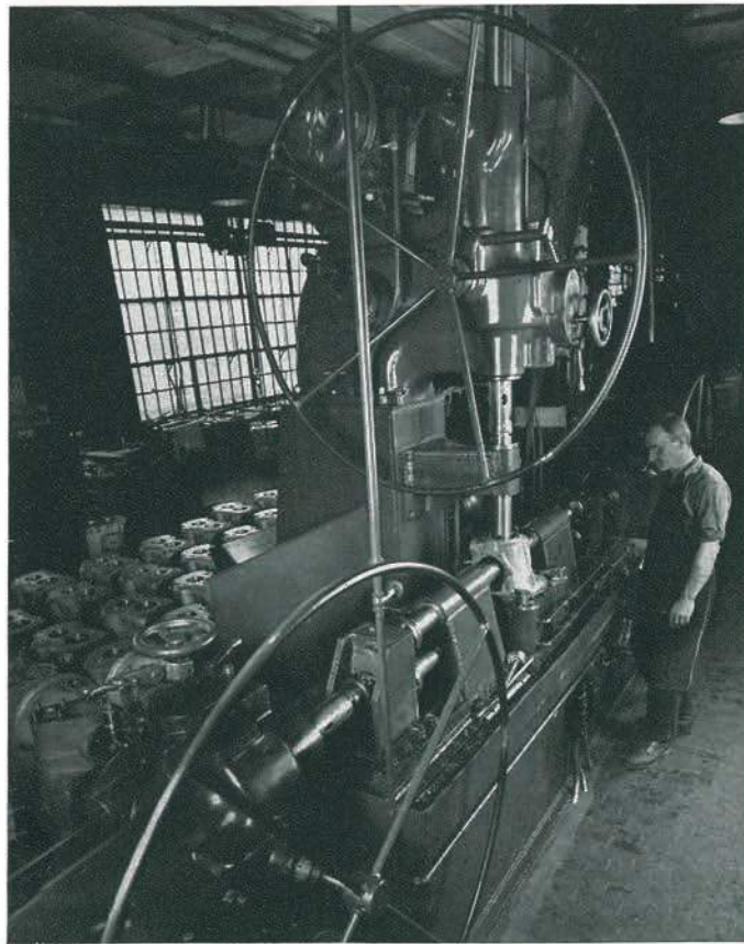
Accuracy of bores in rear axle gear carrier insures exact alignment of driving gears. Because of the great rigidity of this machine Mack holds this accuracy within a half-thousandth inch.
