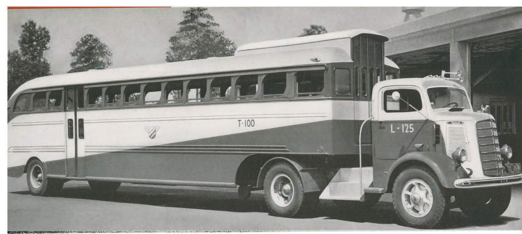
This special tractor-bus carries as many as 59 soldiers on its hourly trips between Ft. Benning and Columbus, Ga. Nine more of the same type have been ordered by Howard Bus Lines.
