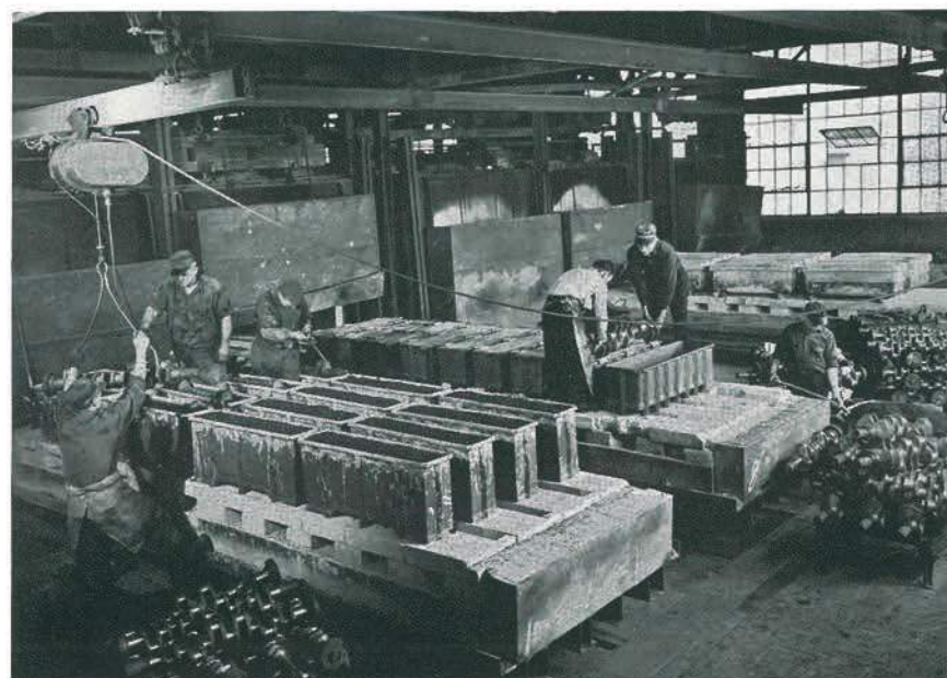
Packed in charcoal- filled boxes Mack crankshafts are heated in cavernous furnaces for 16 hours. Only genuine pack-carburizing makes possible truly case-hardened shafts.
