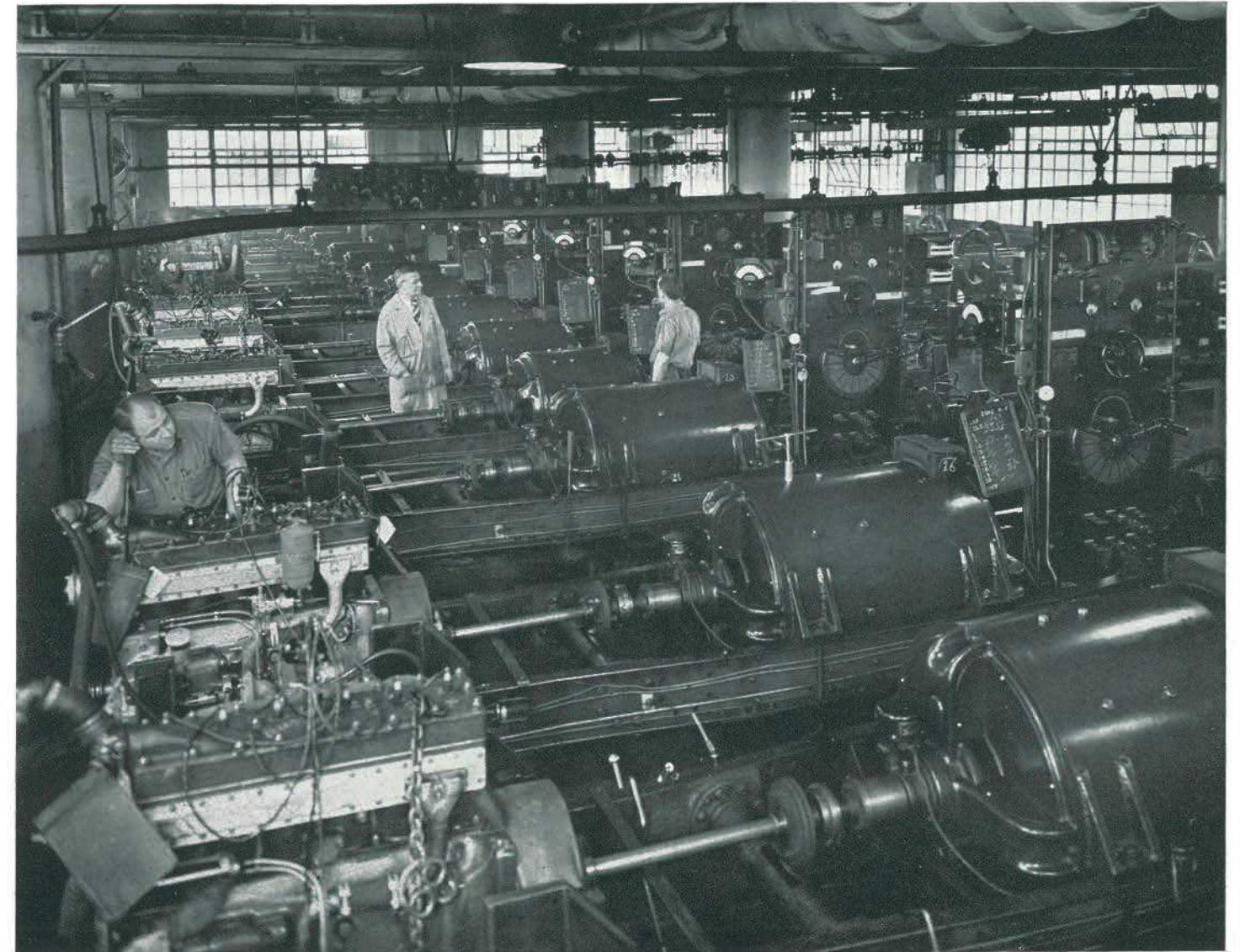
Dynamometer testing of production engines. Mack's dynamometer testing shop accommodates 72 engines at a time. Engines are given two exhaustive tests, each of which takes from 6 to 8 hours. Engines operate with regular grades of fuel and are under constant observation throughout the test.
