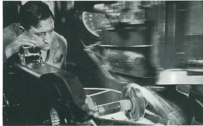
No set of Mack timing gears has ever worn out. Mack makes them tough by case-hardening, then generator-grinds the teeth as shown here for utmost durability and perfect silence.
