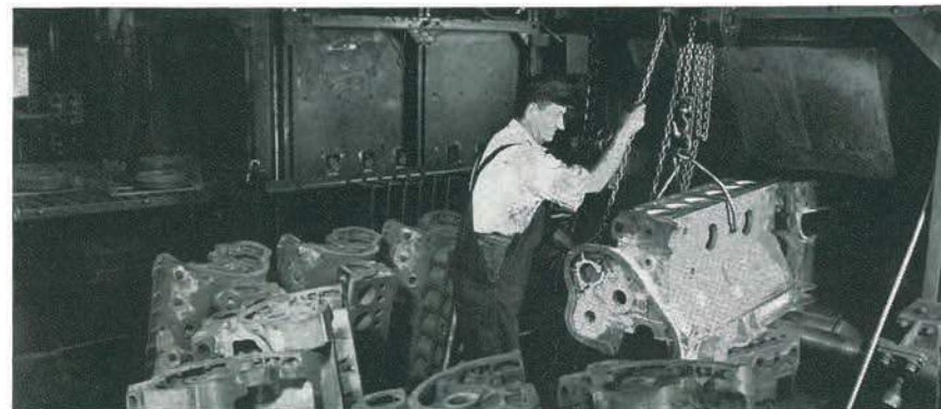
Mack cylinder blocks keep their shape. Shown here, the reason why. Castings enter huge electric furnace for 12 hours of heat treatment. This exclusive process relieves casting strains, prevents distortion.
